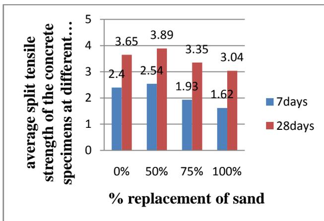
Average Split tensile Strength of Concrete with Quarry Rock Dust in M40 Grade.
