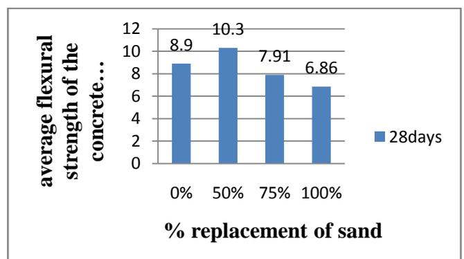
By this table and graphs shows that there is an increase in compressive strength, split tensile strength, flexural strength with 0%, 50%, 75%, 100% replacement of sand with quarry rock dust and it decreases with after 50% replacement in both M30 and M40 grade of concrete.
