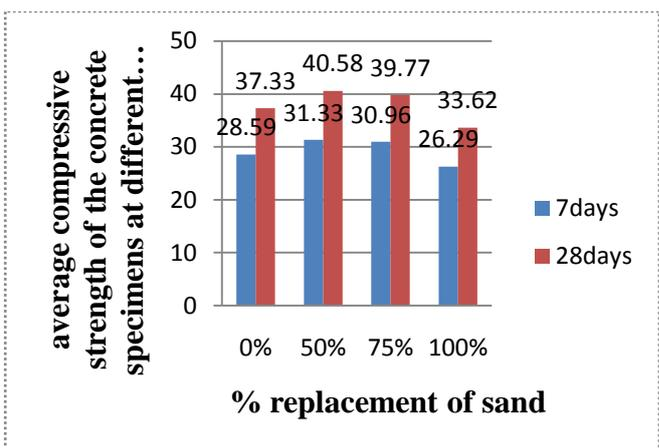
Average Compressive Strength of Concrete with Quarry Rock Dust in M40 Grade.
