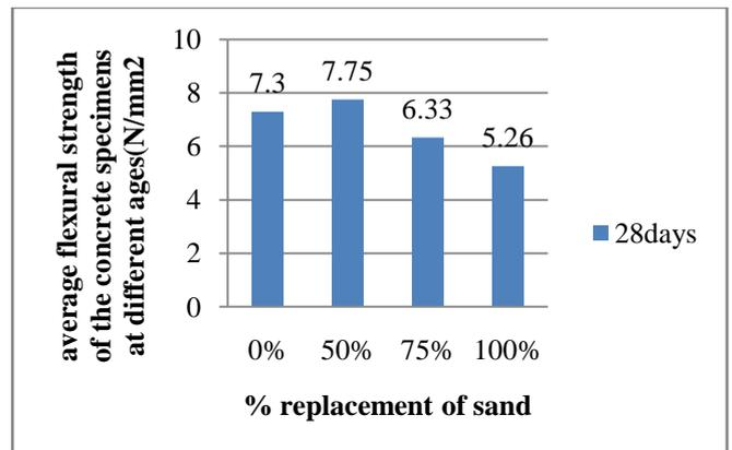
Average Flexural Strength of Concrete with Quarry Rock Dust in M40 Grade.
